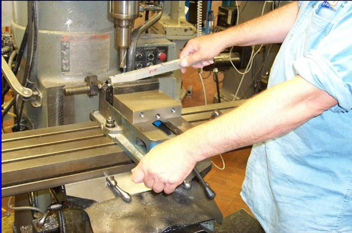
**Before running the machine it should be tried manually to make sure it is clear for cutting.**
