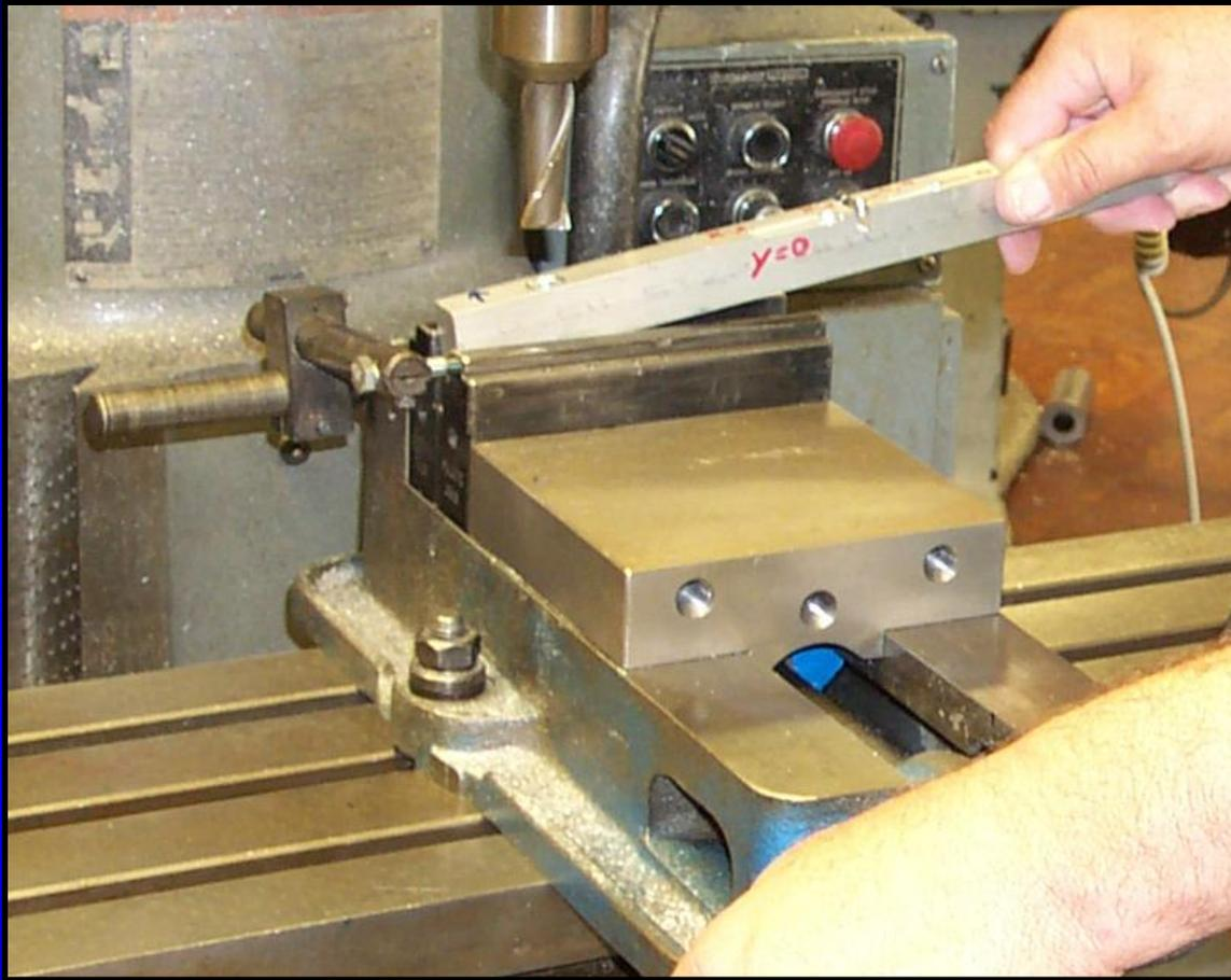
**Make sure workpieces are secure before operating the cutting tool.**
